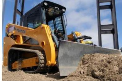
Since the switch to Tier 4 Final engines, there has been a shift in the marketplace, with the popularity of compact track loaders (CTLs) on the rise. For those who prefer a vertical lift model, the Mustang’s 3200VT boast a new vertical lift path lift arms, which have a low-profile rear brace for similar stiffness levels of radial arm models.
