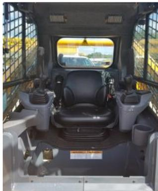
The 3200VT come standard with seat-mounted pilot joystick controls and dual batteries for extra cranking power in cold weather conditions. In the comfortable operator’s station, the joystick controls are mounted to the suspension frame seat, allowing them to move with the operator and reduce fatigue. Controls, armrests, restraint bar and foot pod depth are adjustable. An easy-to-use multi-function display features all the machines vital information
